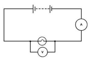
An electric circuit is set up to measure the resistance of one of the lightbulbs. The potential difference is measured to be 12 volts (V) and the current is 50 milliamperes (mA).
